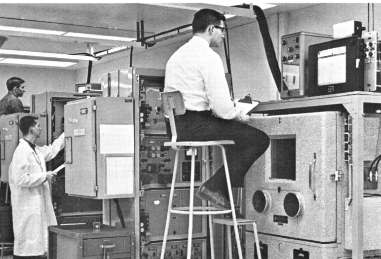
Each MOISTRON System is calibrated prior to shipment using actual samples of the customer's product.
