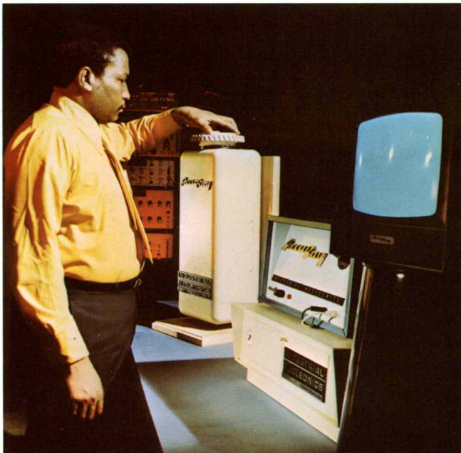
22 AccuRay KET system was further developed to provide instantaneous visual readout of defects or flaws in materials.
