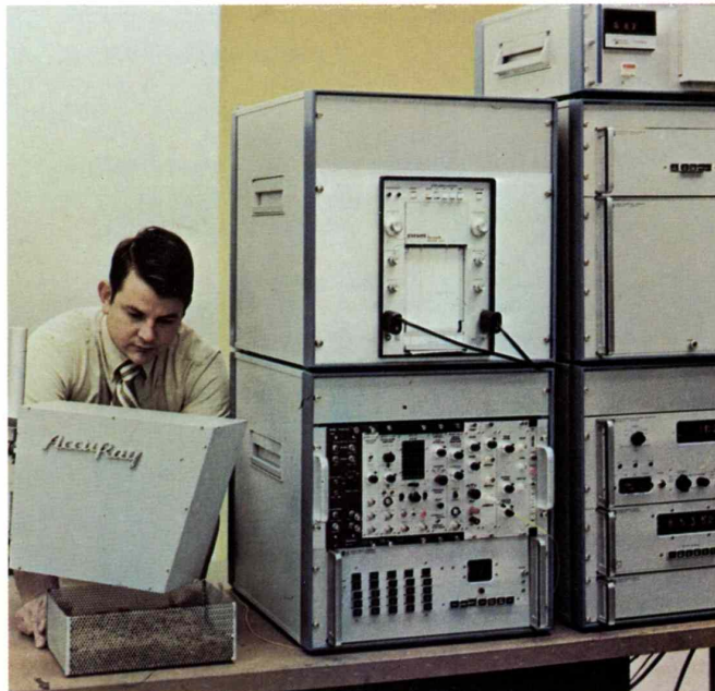
A new infrared measuring principle is employed to determine moisture in tobacco.
