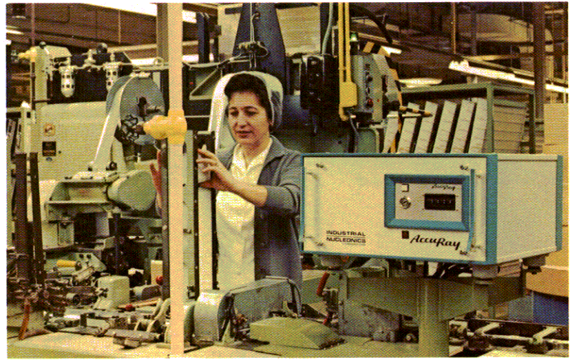
In the packing department of this Canadian manufacturer, new AccuRay system monitors quantity of each brand packaged for shipment.
