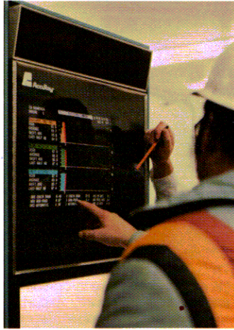
The production and quality information and process control provided by AccuRay 6000 MICRO Sawmill Systems (top left) yield annual savings of nearly $1 million. The most popular of the system's modules, the AccuRay Trimmer Optimizer (bottom right), measures and controls each board cut from the log to maintain the maximum amount of saleable wood.
