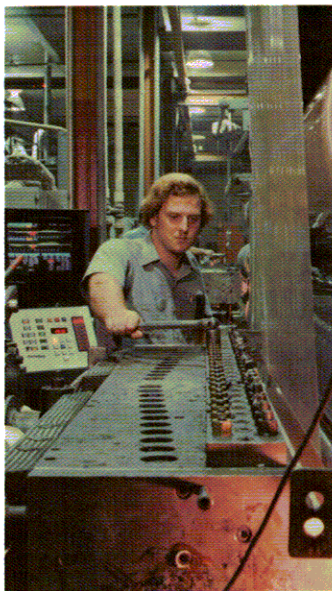
AccuRay systems reduce variations in the extrusion of plastic sheet and film by up to 85 percent. The systems proprietary sensors and controls are also used for specialized extrusion coated aseptic packaging of consumables such as fruit juices, dairy products and dessert puddings.
