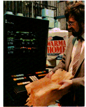
Sensors housed in the U-Frame scanner (left) measure the components of fiberglass insulation as it is being manufactured and relay this data to a computer console (above) for automatic control. Color video reports give operators information about the efficiency and quality of the manufacturing process.
